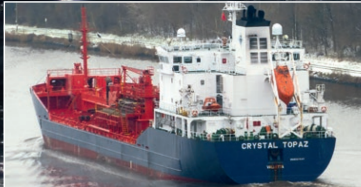
Crystal Topaz 11,340 dwt, length 126 m, 5,406 kW, 15 kn, built 2006 by INP Ulsan, ice class 1A
