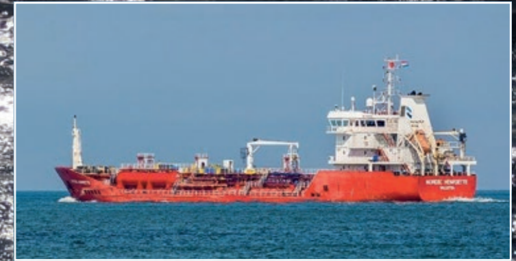
Nordic Henriette 5,600 dwt, length 105.5 m, 2,999 kW, 14.5 kn, built 2008 by Istanbul SY Tuzla, ice class 1A
