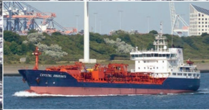
Crystal Amaranto 9,931 dwt, length 126.75 m, 5,280 kW, 12.7 kn, built 1999 by CN Fratelli Orlando Livorno, ice class 1A
