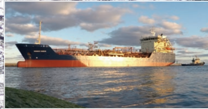
Nordic Nadja 5,764 dwt, length 99.75 m, 2,640 kW, 13 kn, built 1996 by United Naval de Levante Valencia, ice class 1B
