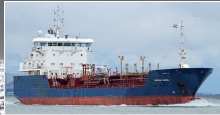
Nordic Nora 5,811 dwt, length 99.75 m, 3,589 kW, 13 kn, built 1997 by United Naval de Levante Valencia, ice class 1 A
