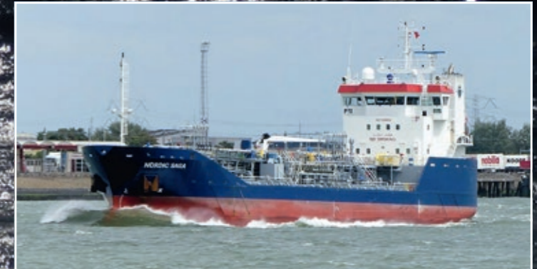
Nordic Saga 4,078 dwt, length 89 m, 1,980 kW, 12.5 kn, built 2007 by Volharding Hoogezand, ice class 1B
