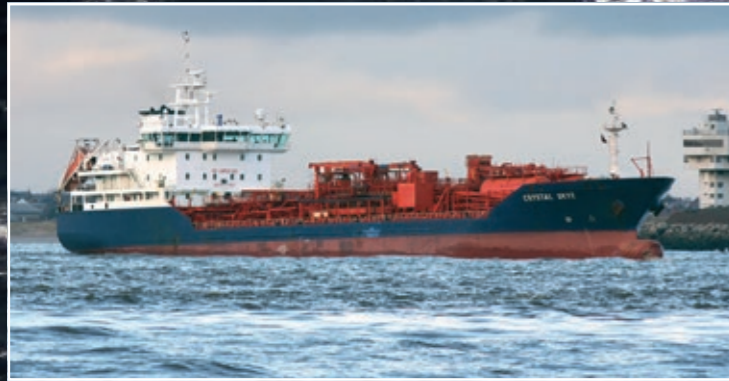
Gisela Essberger (Crystal Sky), 9,554 dwt, length 125 m, 7,178 kW, 14.5 kn, built 1998 by CN Fratelli Orlando Livorno, ice class 1A
