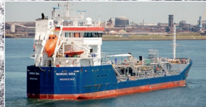
Nordic Sira 4,054 dwt, length 89 m, 1,980 kW, 12.5 kn, built 2006 by Volharding Hoogezand, ice class 1B
