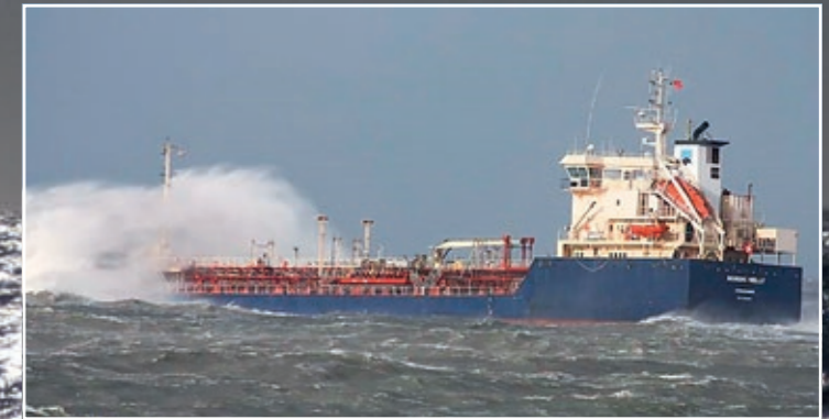
Nordic Nelly 5,767 dwt, length 99.75 m, 2,640 kW, 13 kn, built 1997 by United Naval de Levante Valencia, ice class 1A
