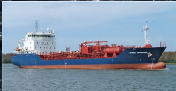
Nordic Marianne 6,228 dwt, length 99.95 m, 5,221 kW, 14 kn, built 2005 by Sekwang HI Mokpo, ice class 1A
