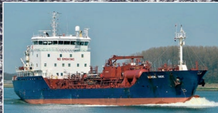
Nordic Inge 6,203 dwt, length 100 m, 5,221 kW, 14 kn, built 2005 by Sekwang HI Mokpo, ice class 1A
