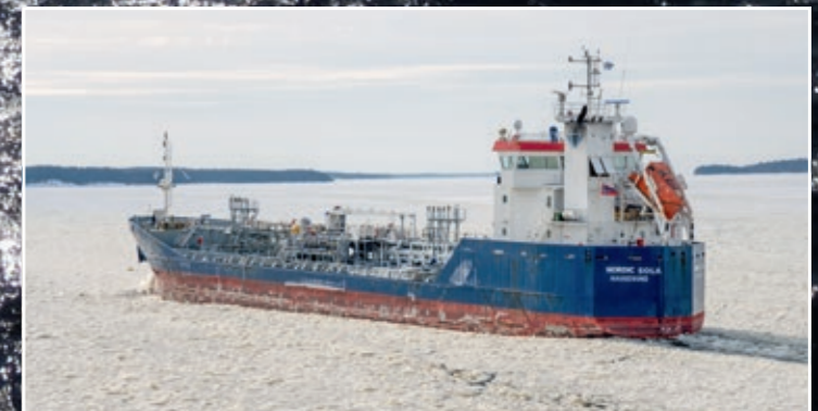
Nordic Sola 4,054 dwt, length 89 m, 1,980 kW, 12.5 kn, built 2008 by Volharding Hoogezand, ice class 1B
