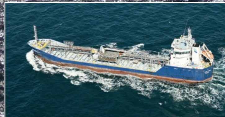
Nordic Sund 4,053 dwt, length 89 m, 1,980 kW, 12.5 kn, built 2007 by Volharding Hoogezand, ice class 1B
