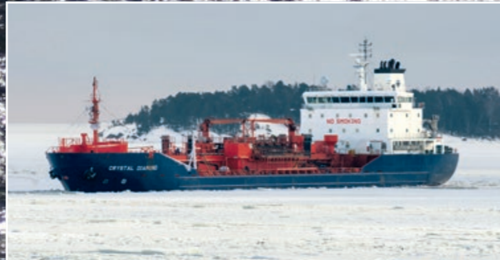
Crystal Diamond 11,340 dwt, length 126 m, 5,400 kW, 15 kn, built 2006 by INP Ulsan, ice class 1A
