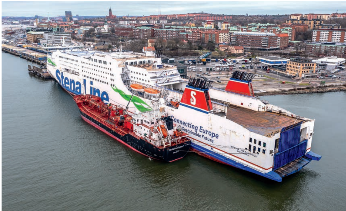
Moored alongside the cargo and passenger ferry "Stena Germanica" (64,039 GRT) in the port of Gothenburg, E&S Tankers' "Stolt Sandpiper" (4,449 dwt) transfers the methanol bunker straight into the ship's fuel tanks
