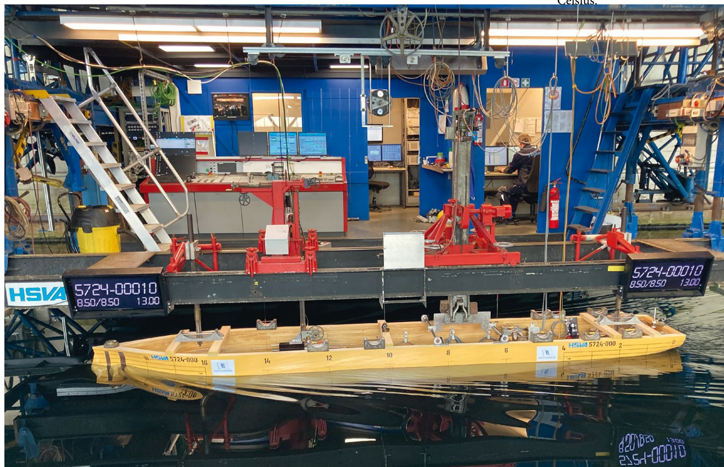
Hullmodel of 13,000 dwt Essberger chemical tanker type in the towing tank of Hamburgische Schiffbau-Versuchsanstalt (HSVA)
