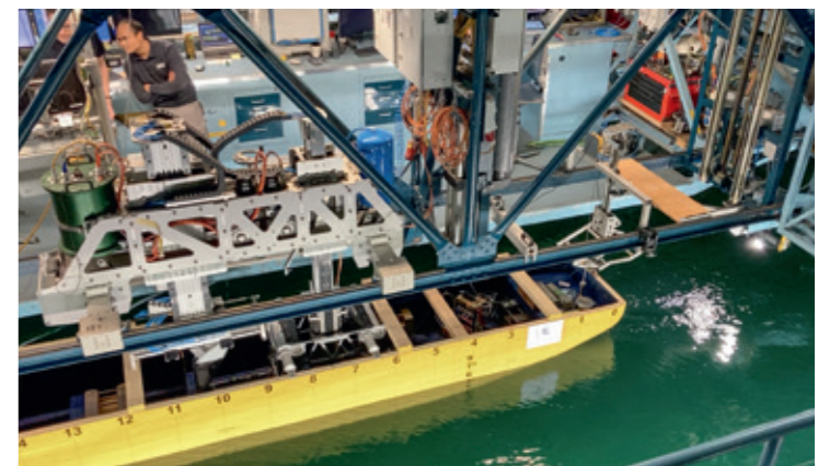
Collecting data in the tank while the model is being pulled through the channel under different stages of load
