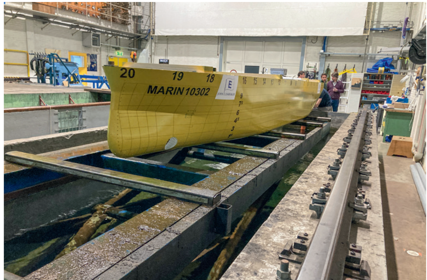
Massive tank test model of new 6,600-dwt chemical tanker at the MARIN institute in Holland. The bulb is integrated into the hull
