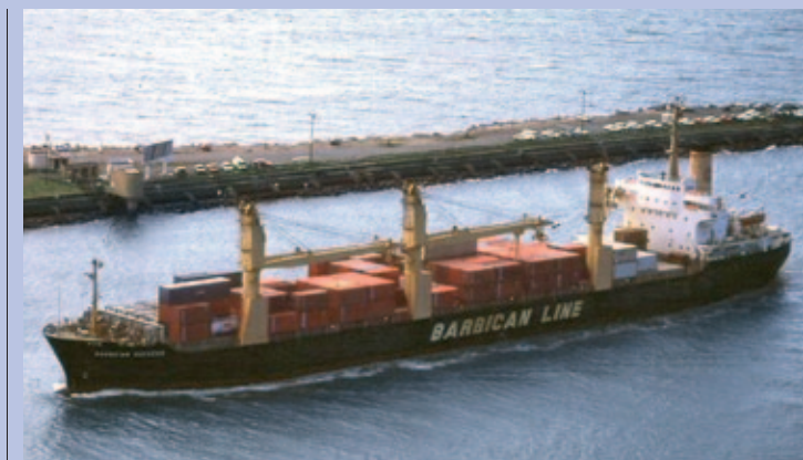
“Barbican Success” (904 TEU, ex-“Frauenfels”) was built in 1973 by Nipponkai Heavy Ind. and later lengthened and turned into a container vessel
