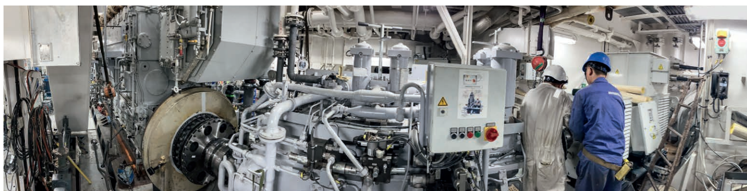
A first look at the heart of the new vessel: the engine room with the MAN dual-fuel propulsion system
