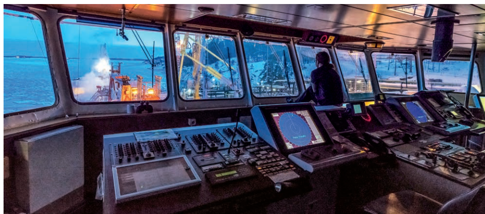
Remote control instruments, screens and various technical devices on the bridge of a chemical tanker. This vessel sails without a traditional steering wheel
