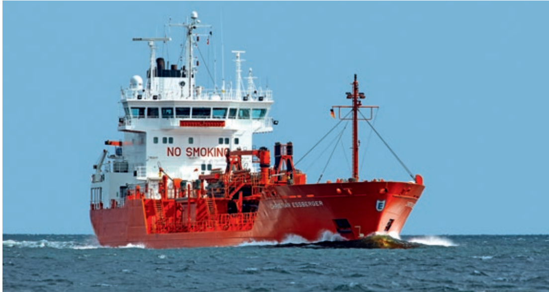
Stainless steel chemical tanker "Christian Essberger" (7,705 dwt, 99 m) steaming along the Baltic in top shape. She was built in 2000 – should she soon be too old to trade?
