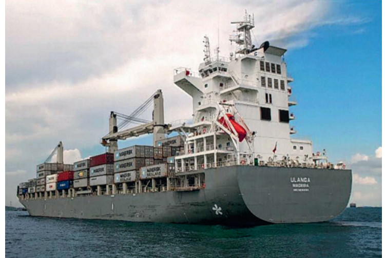
Delivered in 2016 "Ulanga" (2,268 TEU) is one of Essberger Dry Cargo's state-of-the-art container ships. With her 500 plugs for reefer containers and three 45-ton on-board cranes she is a perfect vessel for outport feeder operations
