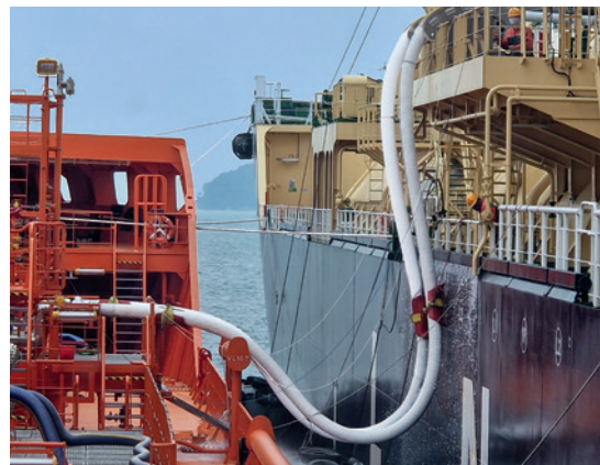
Two pipelines connect both vessels. They are attached to the LNG manifold on the deck of "Liselotte", just below the tank
