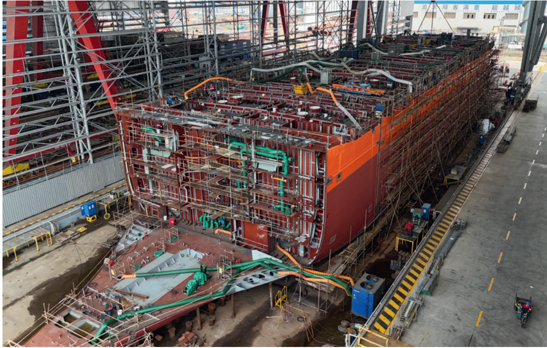
Inside view of the modern shipbuilding hall of Rainbow Shipyard. The "Ann-Mari Essberger" hull is almost assembled but still missing the stern part and superstructure. Thanks to the sheltered dry dock, bad weather is kept out
